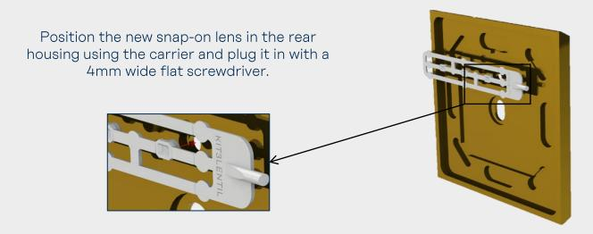
Remove the carrier by rotating it, while holding the lens in its housing.
