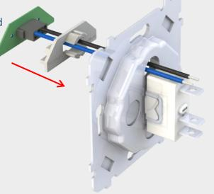
Fold the cables neatly aside as they leave the terminal block to keep the area clear and to avoid pressure on the panel.
